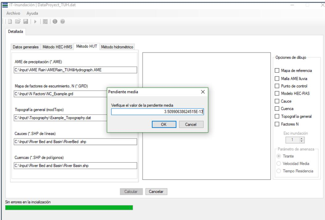
Figure 34. Basin mean slope value window – TUH method
