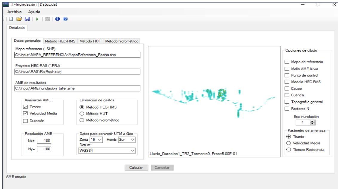
Figure 27. AME Result in the graphic interface – HMS method
