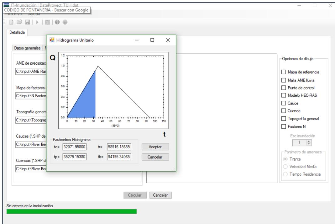
Figure 35. Unit hydrograph parameters window – TUH
