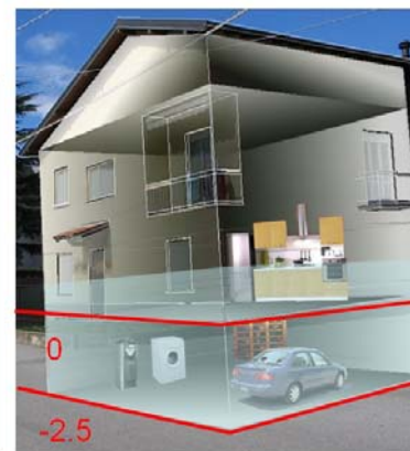
Figure 4.20: Percentage of losses of the total value of the property due to increasing flood level, starting at - 2.5 when basement is flooded. (Source: Fabio Luino)
