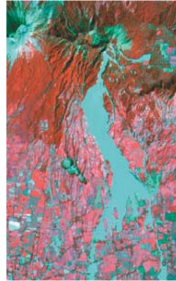
Figure 2.9. SPOT satellite optical image of a volcanic mudflow in Nicaragua (20m resolution).
