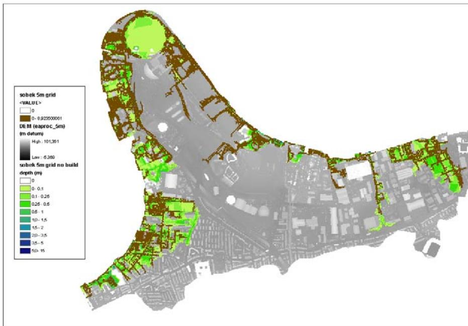
Figure 3.11 Flooded area for the 5m grid with buildings (brown) or without buildings (green), computed with the SOBEK model.
