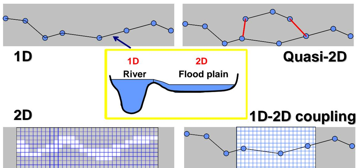
Figure 1.1 Types of numerical models used for inundation modelling
