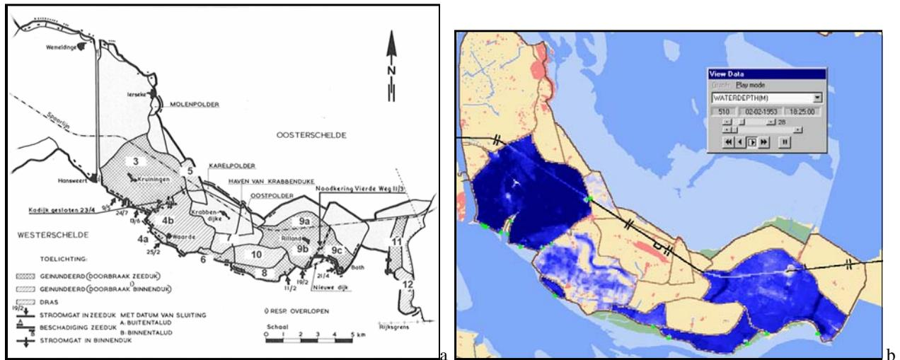
Figure 3.1 Observed flooding patterns during the flood of 1953 (a) and water depths computed with SOBEK (2D)(b) (source figure a: Rijkswaterstaat and KNMI, 1961)
