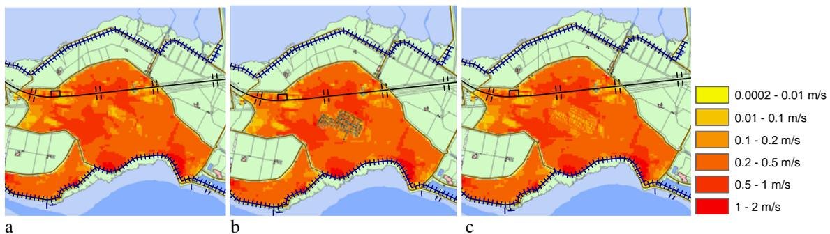
Figure 3.7 Flow velocities computed with a coarse grid (a), a finer grid and solid buildings (b) and a finer grid with very high roughness values representing buildings (c)
