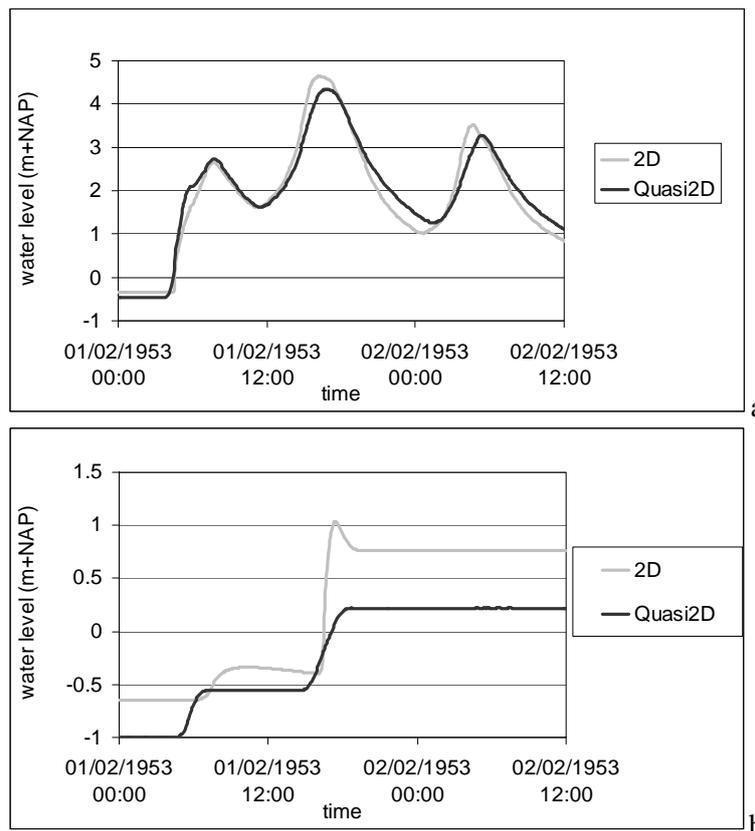
Figure 3.3 Water levels (m +NAP) computed with the 2D and quasi 2D application of SOBEK for polder 3 (a) and polder 4b (b) (for locations see Figure 3.1a)
