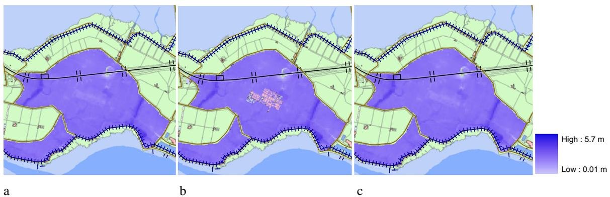
Figure 3.6 Water depths computed with a coarse grid (a), a finer grid and solid buildings (b) and a finer grid with very high roughness values representing buildings (c)
