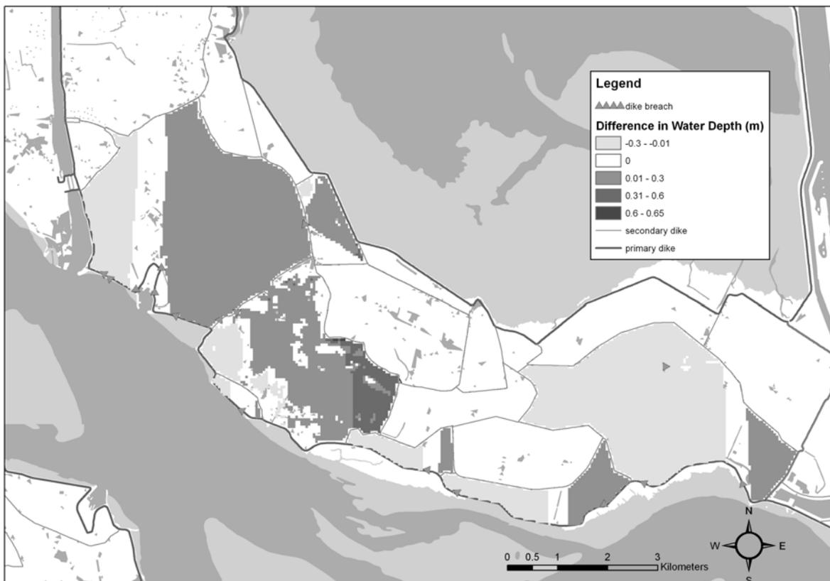
Figure 3.8 Difference in water depth (m.) between the simulation with wind force 10, direction west, and the simulation without wind
