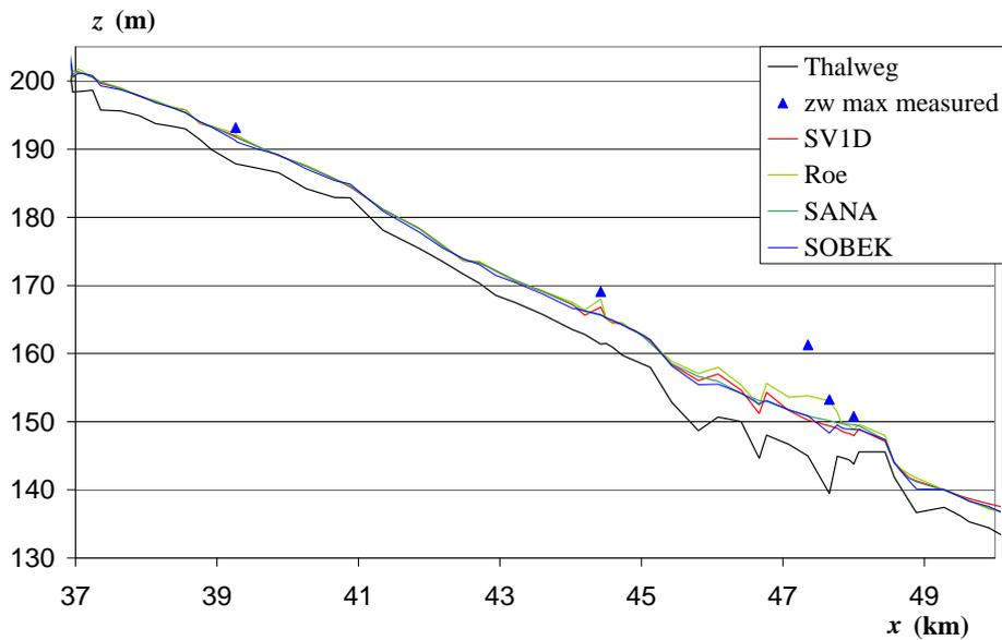
Figure 3.16 Simulated and measured maximum water levels between  $x = 37$  km and  $x = 50$  km
