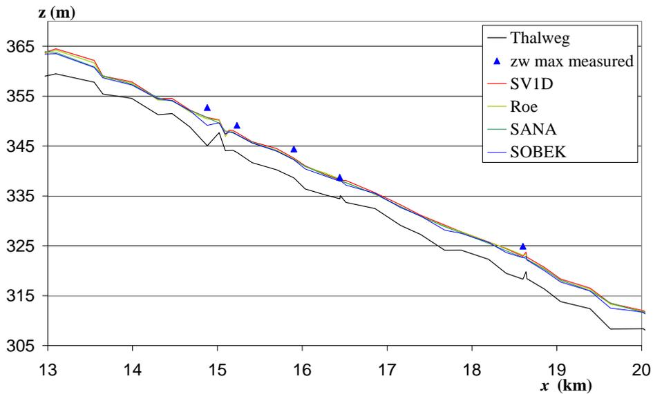
Figure 3.13 Simulated and measured maximum water levels between  $x = 13$  km and  $x = 20$  km
