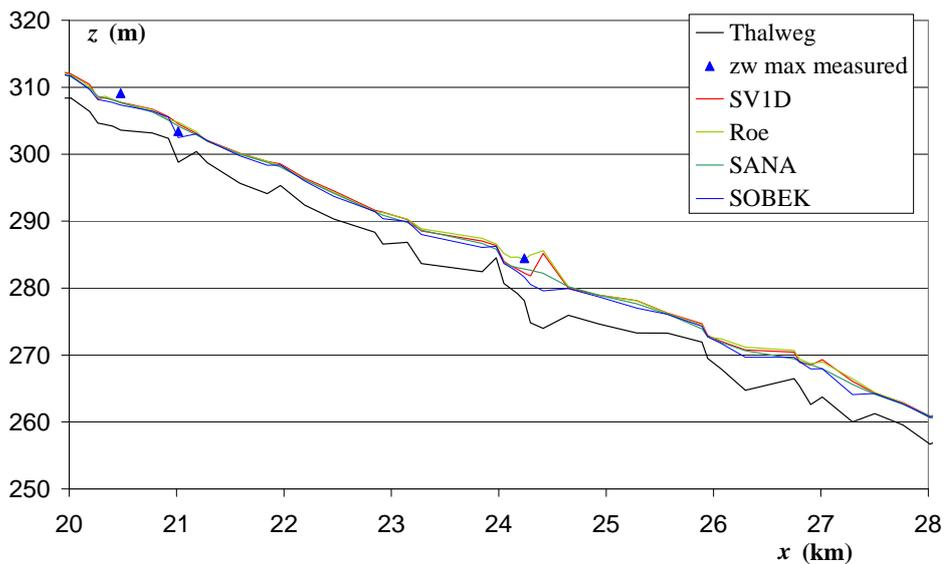
Figure 3.14 Simulated and measured maximum water levels between  $x = 20$  km and  $x = 28$  km
