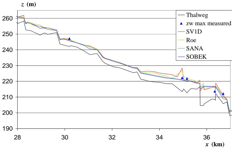
Figure 3.15 Simulated and measured maximum water levels between  $x = 28$  km and  $x = 37$  km
