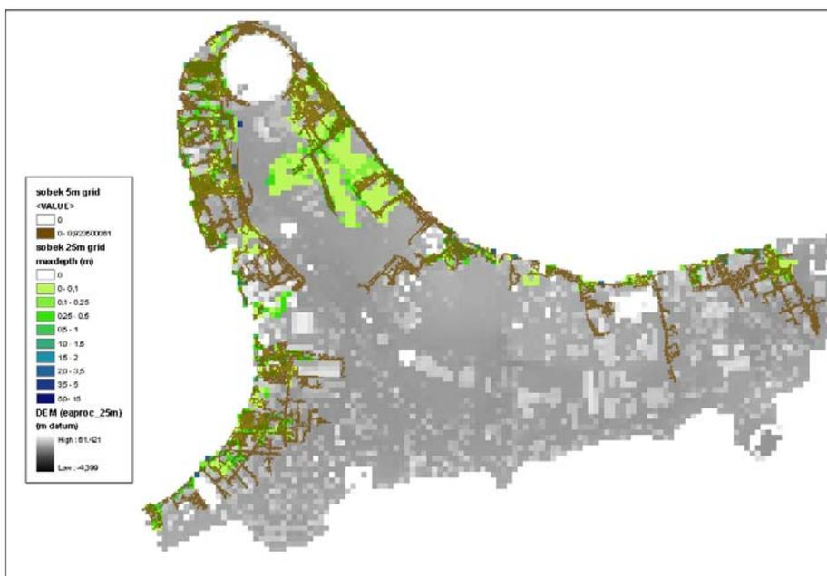
Figure 3.10 The flooded area in the 5 and the 25m grid cell size, computed with the SOBEK model. The 5m grid is on top and represented by the brown colour. The 25m grid is in green, which represents the calculated water depth.
