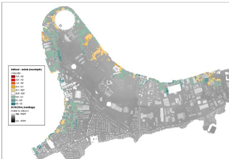
Figure 3.9 Difference in maximum water depth computed with SOBEK and LISFLOOD-FP (blue means that LISFLOOD is deeper, yellow or red means that SOBEK computes larger depths)
