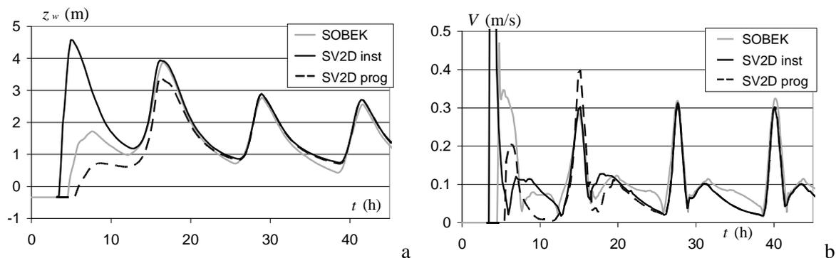
Figure 3.2 Computed results in polder 3 (Figure 3.1a): (a) water level and (b) velocity
