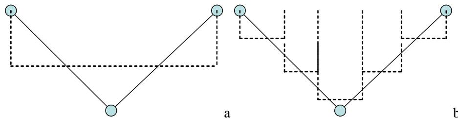
Figure 3.17 Schematisation of yz-cross sections (blue dots are yz points given by the user, the bold line represents the actual cross section and the dotted line the cross section used by the model)
