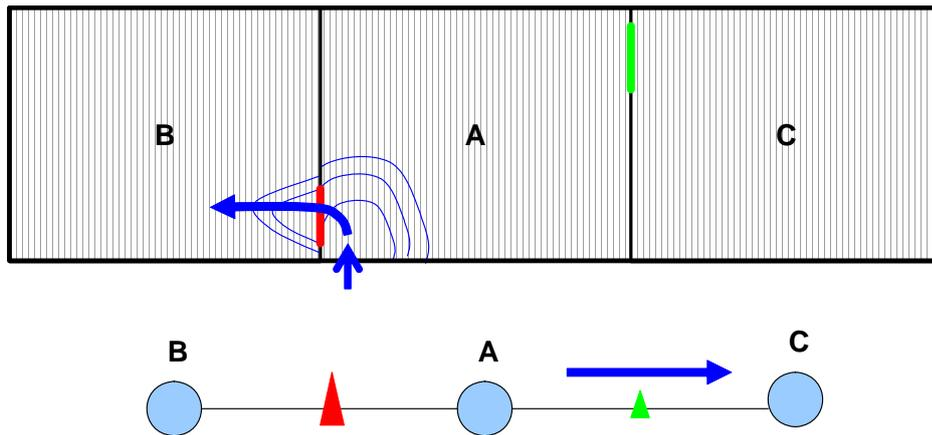
Figure 3.4 Schematisation of 3 polders in 2D (upper half) and quasi 2D (lower half). Red and green lines represent low sections in secondary dikes between the polders. The green section is lower than the red section.
