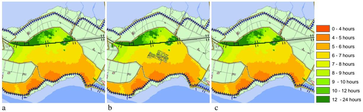
Figure 3.5 Moment of first inundation computed a coarse grid (a), a finer grid and solid buildings (b) and a finer grid with very high roughness values representing buildings (c)
