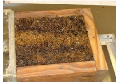
Fig. 14: Vetiver roots after erosion testing
