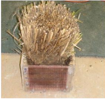
Fig. 13 Vetiver stems after erosion testing
