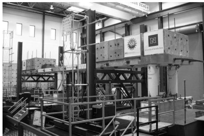
Figure 8: Bridge model prior to testing.
